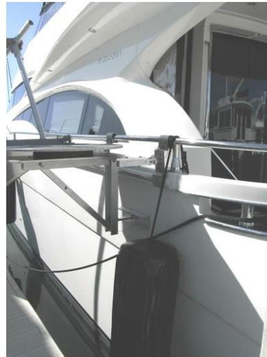
Our vessel swivel platform-boarding mount can be used with our any of our fixed length ramps This mount will allow you to support our fixed length ramp from either side of your vessel or the transom and position the ramp forward, aft, side-to-side or straight out. (180 degrees swivel).
